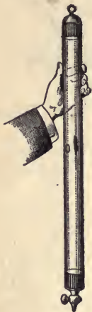
FIG. 37.—Bodies Fall Alike in a Vacuum.
